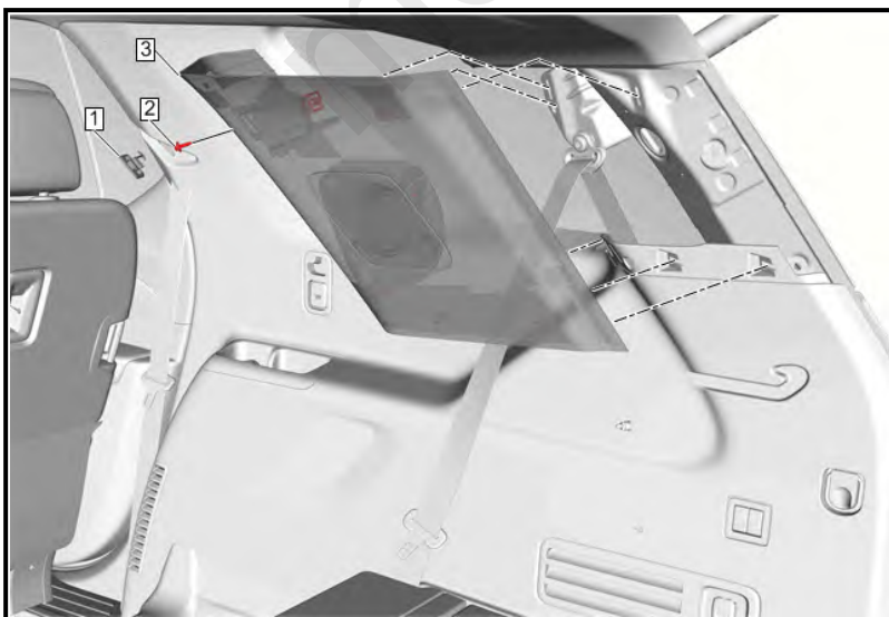
Body Rear Corner Upper Garnish Molding (3) - Remove [2x] - Body Rear Corner Upper Garnish Molding Replacement
