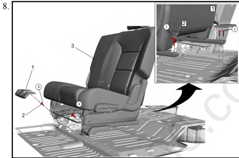
Rear Seat-60% (3) - Install - Rear Seat Removal and Installation (60%) .
