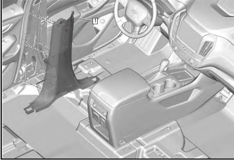
Center Pillar Lower Trim Panel (1) - Install - Center Pillar Lower Trim Panel Replacement
