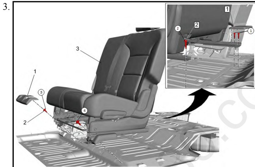
Rear Seat-60% (3) - Remove - Rear Seat Removal and Installation (60%)
